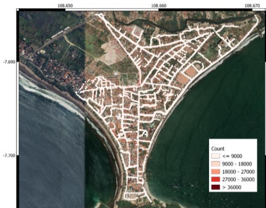
Figure 3. Congestion severity map — indicates how severe the congestion is on a specific road. The higher the number (dark red), the more severe the congestion was.
